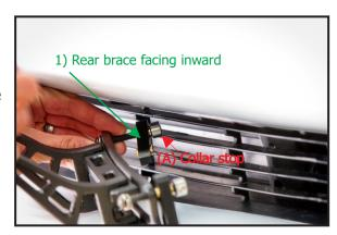
2) Align the rear brace vertically, insert bolt into rear brace hole (split lock washer, then flat washer), then using the included 5/32 hex key, hand-start the 1/4-20 bolt into the threaded insert. Check for center alignment before securing all 4 bolts without over-torquing.
