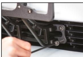
3) Secure your license plate using a Phillips screwdriver with 4 of the #10 x 3/8" screws.
